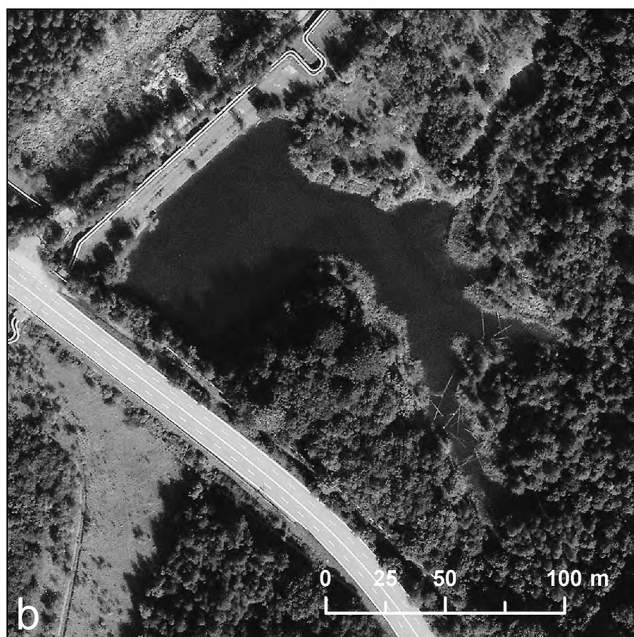
Fig. 4 (a, b) Submerged ground subsidences (a) in an aerial photo from 1947 (© MO ČR/GeoSI AČR) and (b) in an aerial photo from 2009 (© GEODIS BRNO, spol. s r. o.) in Karviná-Doly mining area
