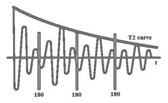
Figure 2. The T2 curve created as a result of the pulse sequence 90°-180°-180°-180°. It shows that the individual echoes are getting gradually lower signal intensity
