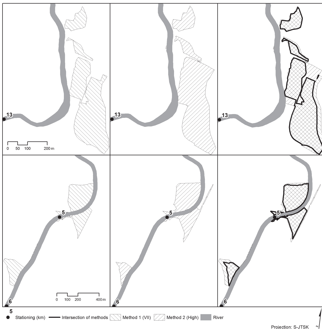
Fig. 4 Differences in areas of flood risk categories (VII and High) identified by both methods.
