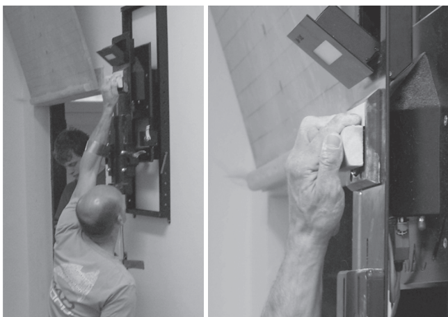
Figure 1. Special dynamometry – 3D-SAC for measurement finger flexor strength, body and finger position during the tests
