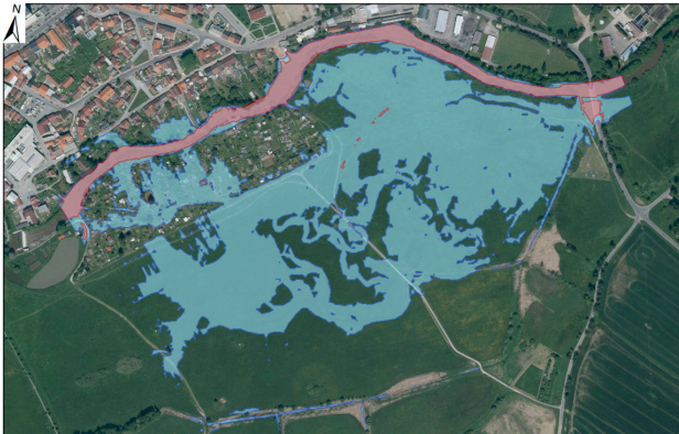
Fig. 22 Comparison of inundation areas at discharge Q_1 at the Úhlava River site.
