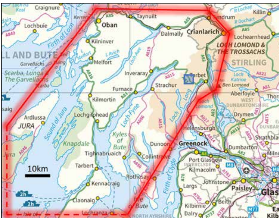
Fig. 4 A relatively small debris flow event (blue rectangle) closed the A83 at the Rest and be Thankful in October 2007; the vulnerability shadow that was cast (bounded in red) was extensive (Winter 2014a; 2014b). See Figure 1 (1b) for the event location in the wider geographical context. (Image based on OS Route Planner 2016 Map. © Crown Copyright. All rights reserved Scottish Government 100020540, 2019.)
