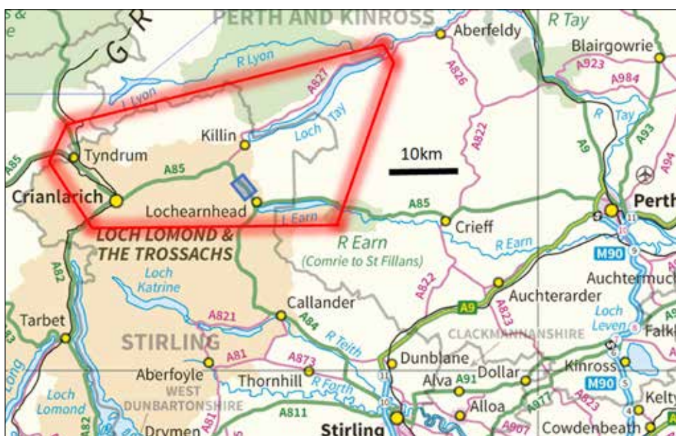
Fig. 10 Two debris flow events (blue rectangle) closed the A85 in Glen Ogle on 18 August 2004; the vulnerability shadow that was cast (bounded in red) was limited by the reasonably good range of alternative routes in the area. See Figure 1 (3) for the event location in the wider geographical context. (Image based on OS Route Planner 2016 Map. © Crown Copyright. All rights reserved Scottish Government 100020540, 2019.)
